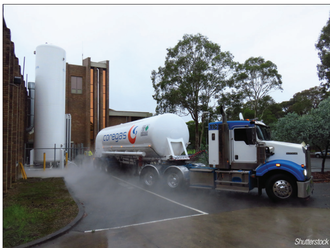
FIGURE 2. Merchant products are liquefied gases that are trucked and sold by industrial gas suppliers to third parties
